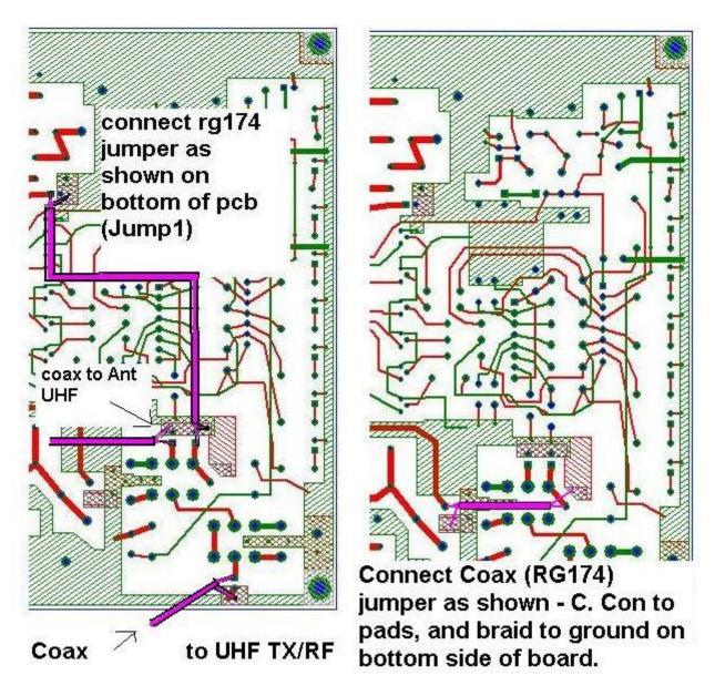
You must install 2 RG174 coaxial jumpers on the bottom side of the PCB. The center conductor connects to the respective pads and the braid to the ground plane. Two additional RG174 or equiv. cables are attached to the top side of the pcb. These cables connect to the chassis mount UHF connectors. You must also decide on the wire jumper settings. See page 1 of the schematic. Make thes jumpers from solid wire #16-18 awg.
