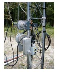
When Whitey, K1VV, mentioned recently that he had to fold his Rohn 25 tower over to service his rotor, I cautioned him to be careful with that winch. Whitey sent me a photo of what I thought was a really clever idea. He keeps an extra winch cable connected to the foldover section, which attaches to a power winch that he installs temporarily in parallel with the normal manual winch. Rather than leave it out in the weather, the power winch is removed when the job is done.
