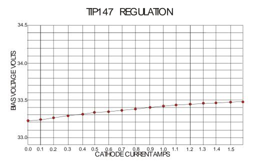
The TIP147 circuit seems to have a bit better shunt regulation performance than the MOSFET version. Impedance of the TIP147 design was about 0.2 ohms at 1 amp of current. Possibly the op amp gain in the MOSFET design could be adjusted for
