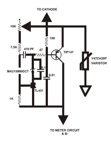
The regulation performance of the TIP147 bias circuit modified for high cathode bias similar to the IRF840 circuit, is as follows:
